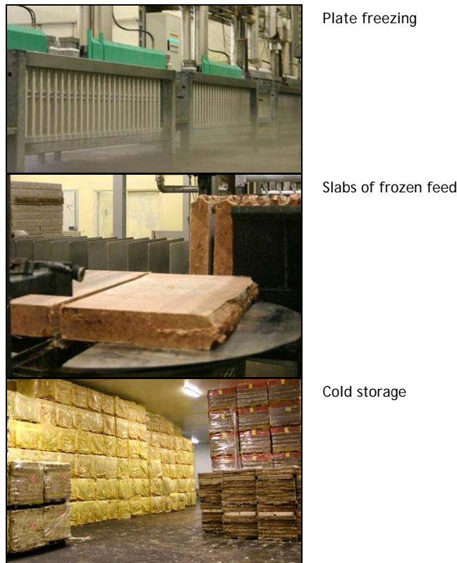
Figure 5 Feed production: plate freezing and storage
